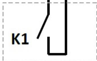
You just need to connect the control connector between the photovoltaic inverter and the appliance's control panel. This connection to the panel must be made potential-free (no voltage). The voltage on this contact causes irreversible damage to the appliance.
